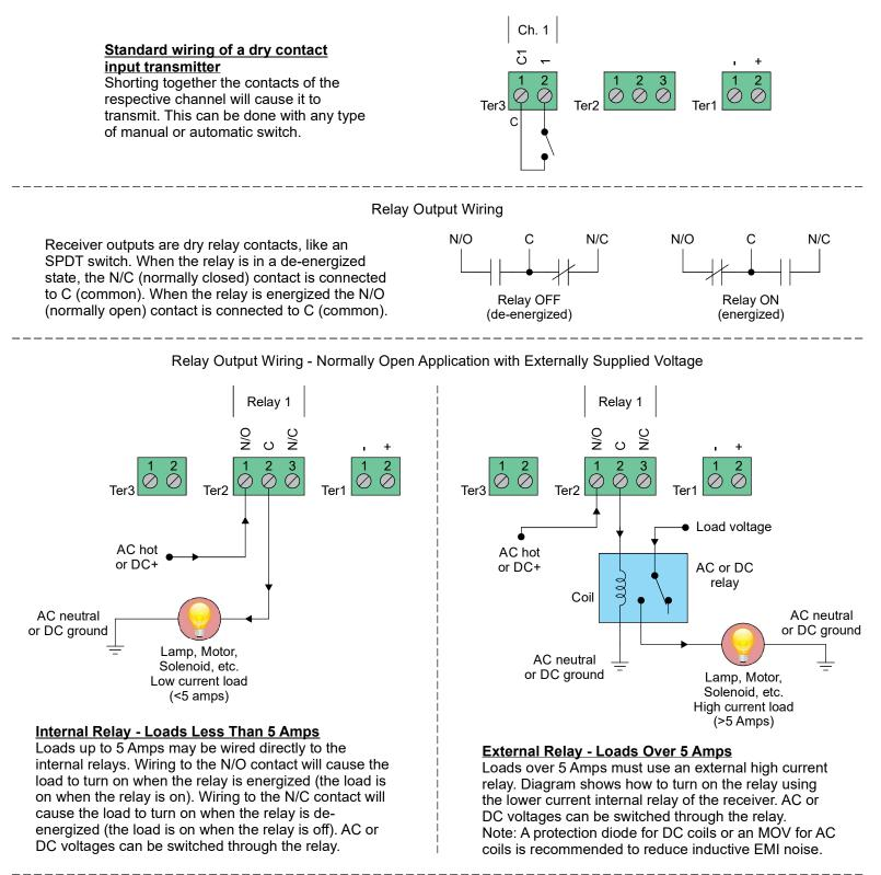
Wiring configurations shown here are examples. The wiring for your application may differ. Call BWI Eagle for assistance or consult an electrician.
