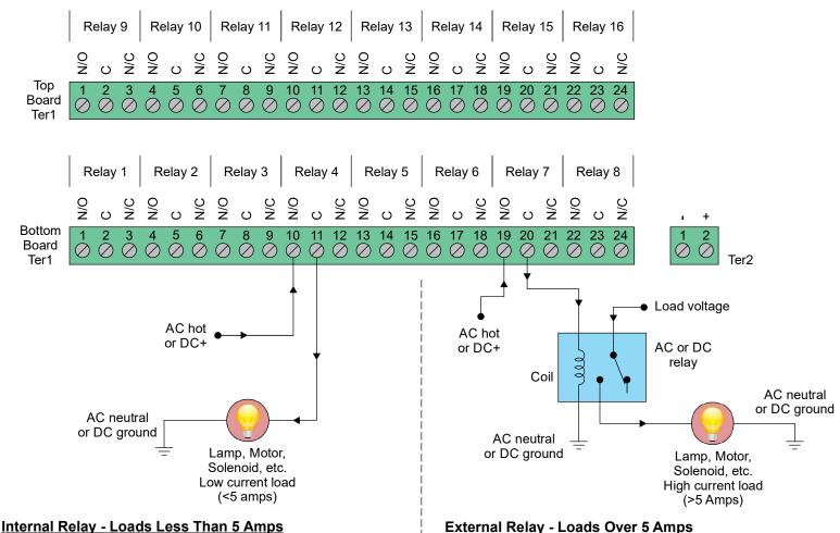
Loads up to 5 Amps may be wired directly to the internal relays. Wiring to the N/O contact will cause the load to turn on when the relay is energized (the load is on when the relay is on). Wiring to the N/C contact will cause the load to turn on when the relay is de-energized (the load is on when the relay is off). AC or DC voltages can be switched through the relay.
